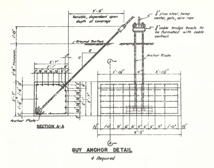
Figure 64. This particular anchor plan is for the standard timber lookout tower, CT-1 series, in the 119 feet version. Anchor plans for other types were very similar.
